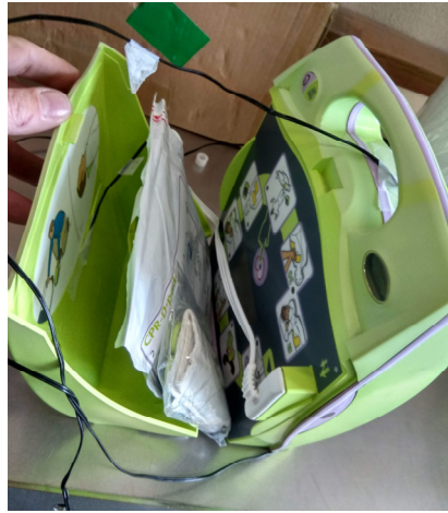
Figure 2-3: Temperature probe 2: top of the AED
